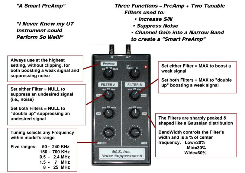
Total Gain = PreAmp (30db) + Filter A (15db) + Filter B (15db) = 60db
